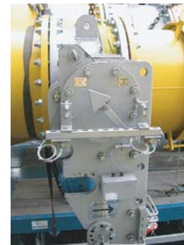
Sub Bypass Valve
